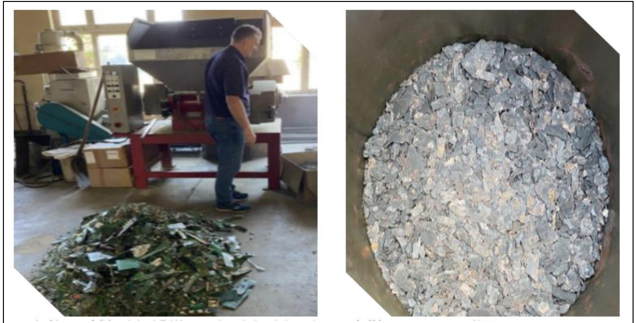
Figure 2: Original E-waste printed circuit board waste and metal rich char (E-waste with plastics removed)
