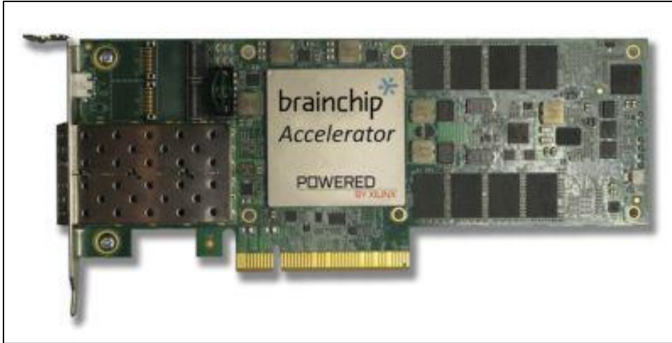
FIGURE 15: BRAINCHIP ACCELERATOR CARD FOR BRAINCHIP STUDIO
