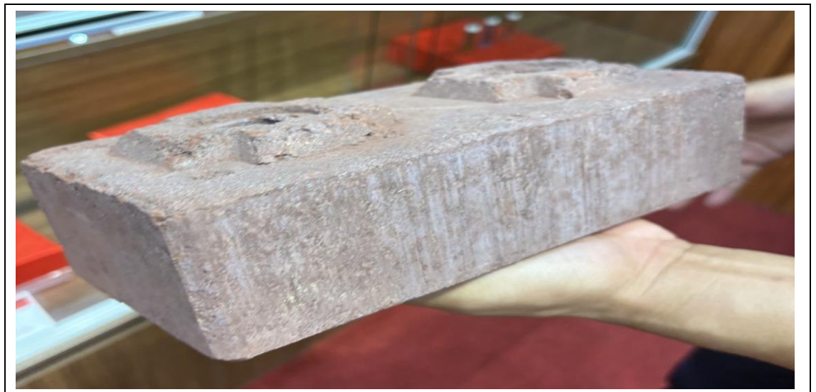
Figure 20: A sample brick produced from residue at the Pilot Plant
