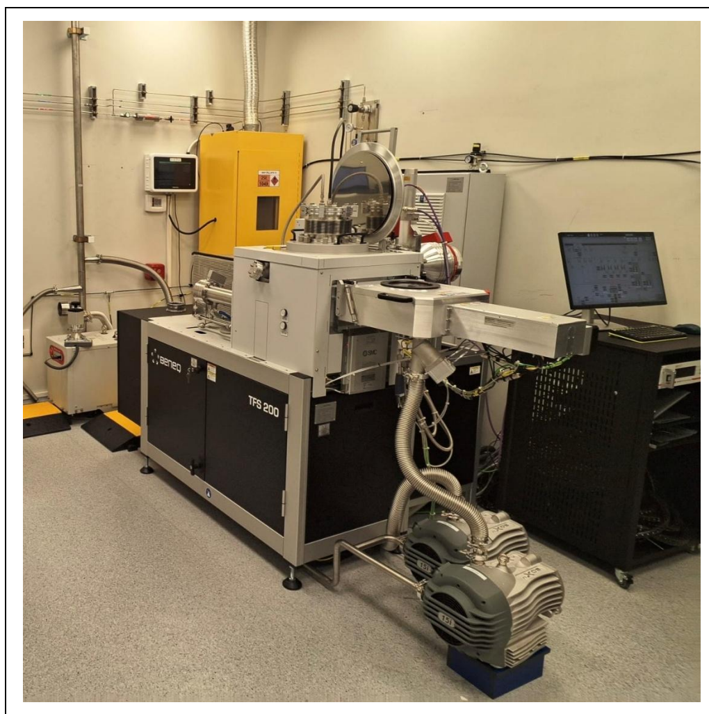
Figure 4: The Beneq TFS 200 ALD system that Adisyn is leasing.
